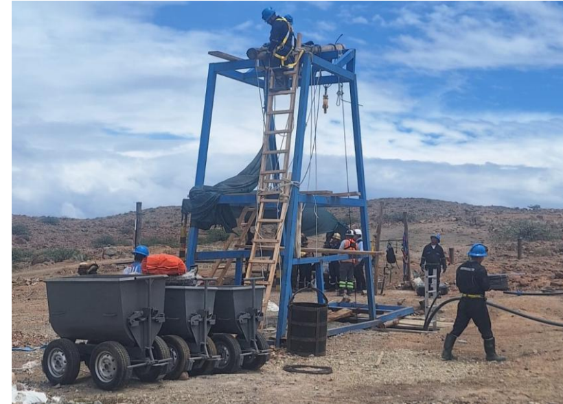
Hoisting and access structures at Bonanza shaft and minecarts to transport vein material (Feb-26)
